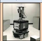
first Shakey the Robot, was developed by Stanford Research Institute in the late 1960s. It was the first machine capable reasoning about actions. combining mobility with artificial intelligence to navigate and interact with its environment.
